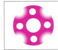
(5) Remove film and observe pressure distribution.
